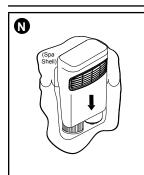
Reinstall the skimmer shield over the filters. Then turn power to spa back on.
